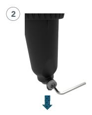
Open the exhaust valve to depressurise the system (5 seconds) and close it again. Use a container to collect drain water
