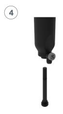
Unscrew the magnet and remove it. Place the magnet on a clean surface.
