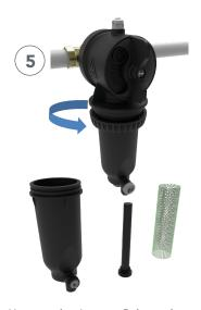
Unscrew the ring nut. Release the body.
