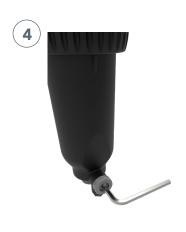
Open the drain and empty the water inside it. Use a container of at least 1 l.
