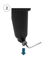
Open the exhaust valve To depressurise the system. (5 Seconds) and close it again. Use a container to collect drain water
