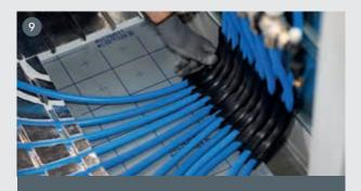
Curve holders prevent the possible crushing of the pipes near their entry into the panel.
