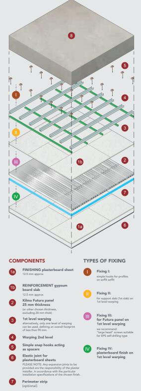
Floor slab (necessarily planar) The Kilma Futura panel **can also be applied to walls**. It can be installed on a masonry or plasterboard wall, then the panel is covered with a sheet of plasterboard or fiberboard. The reduced thickness, quick installation and the use of 16x2 pipes that can be connected directly to the radiant manifold make the Kilma Futura panel suitable for any installation.
