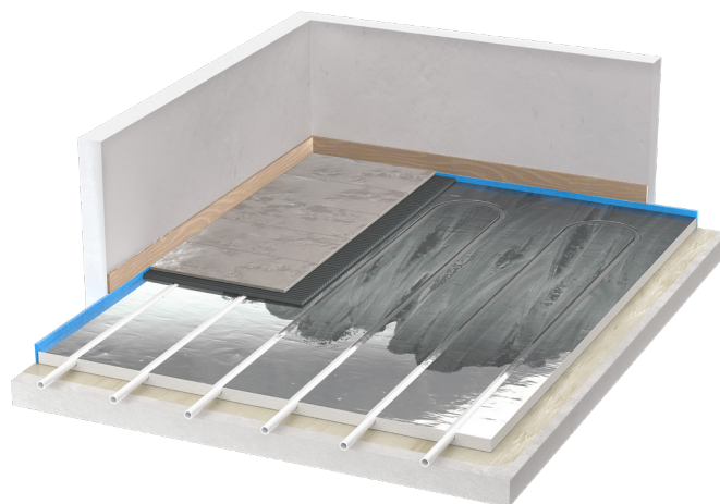
Kilma Futura system with ceramic covering glued directly onto the panel
