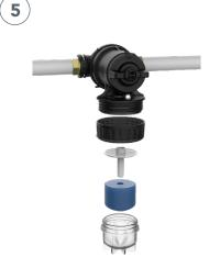
Remove the disc filter, wash well and place the polyphosphates in the beaker **(no powder).**
