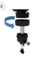
Unscrew the ring nut. Release the body.
