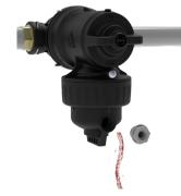
Open the drain. The dirt inside the filter no longer captured by the magnet will be channelled outside by the flow of water in the drain. Use a container of at least 0,5 l.
