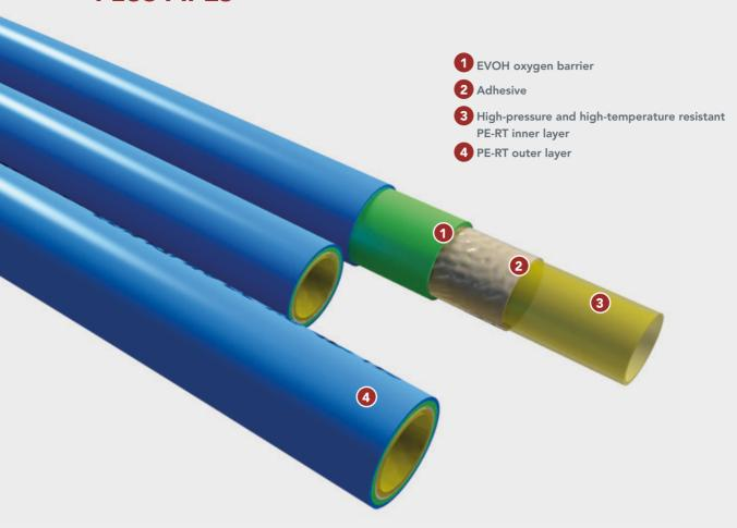
Hi Performance Plus pipes are made of a polymer resin, which has the traditional properties of polyethylene, with the addition of important extra features such as **increased resistance to high temperatures and high pressures.**
