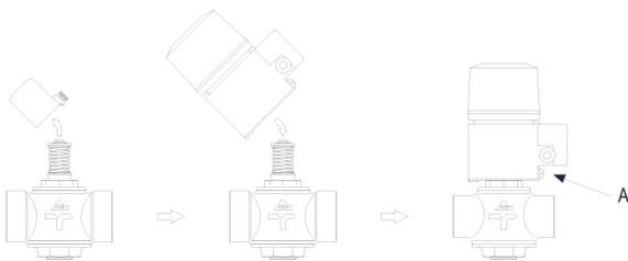
The **zone valves** are supplied, as standard, with the knob for the manual opening and closing control. To automate the valves themselves, simply follow the steps below:
