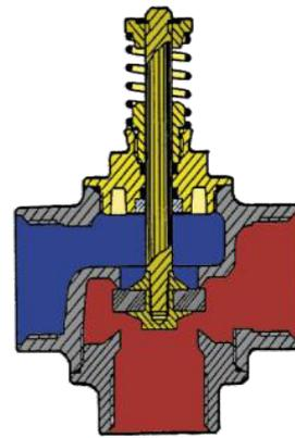
Zone valve **CLOSED** on the straight way. Condition guaranteed **without cap** or with **coupled actuator not powered**.
