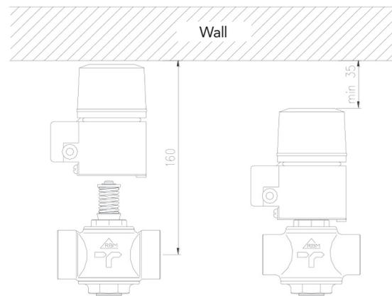
If installing the valves in any zone boxes, according to the type of assembly, leave sufficient space (**35 mm**) at the side or above the actuator to allow the replacement of the same.
