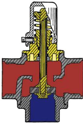
Zone valve **OPEN** on the straight way. Condition guaranteed **with cap attached** or with **coupled actuator powered**.
