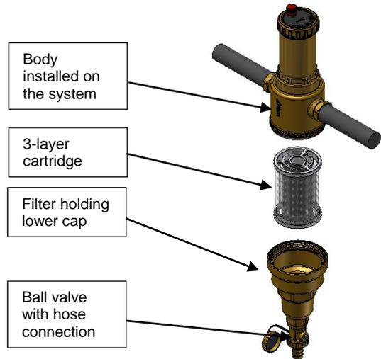
Routine maintenance Filter purgig can be performed with the system running, acting on the ball valve provided with hose connection. It is important **to perform the purge operation** at least **once a year**. In case of first application, perform the first purge after a month.
