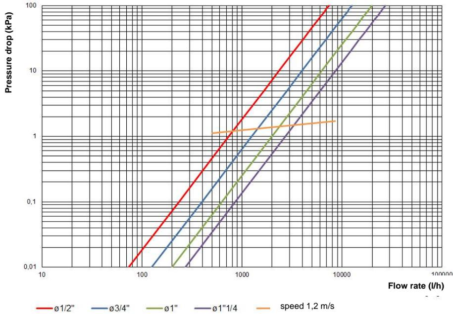
It is recommended to keep the maximum speed of the fluid in the pipe within the value of 1.2 m/s. Higher speeds may impair the proper operation of the air discharge device.
