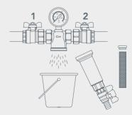
WARNING: During this operation ball valves 1 and 2 must be opened.
