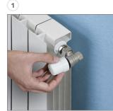
**1.** Remove the manual adjustment handwheel by loosening it anti-clockwise.
