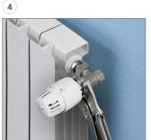
4. Tighten the thermostatic head's knurled metal ring nut onto the valve's body until blocked. Turn the numbered knob a few times after head assembly, from **position "5"** to **position "\*"**, for the parts to settle.
