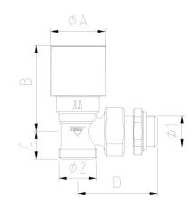
ANGLE VALVE for multilayer, polyethylene, copper pipe
