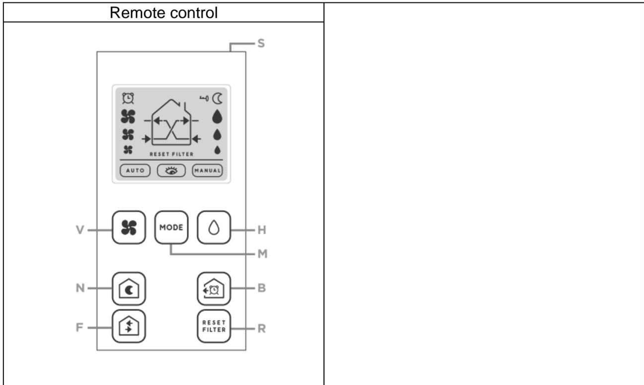
**WARNING (Remote control):** the remote control get into stand-by mode after being inactive for 60 seconds when the icon with key appears on display. To unlock press the button (S) on the upper side of the remote control.
