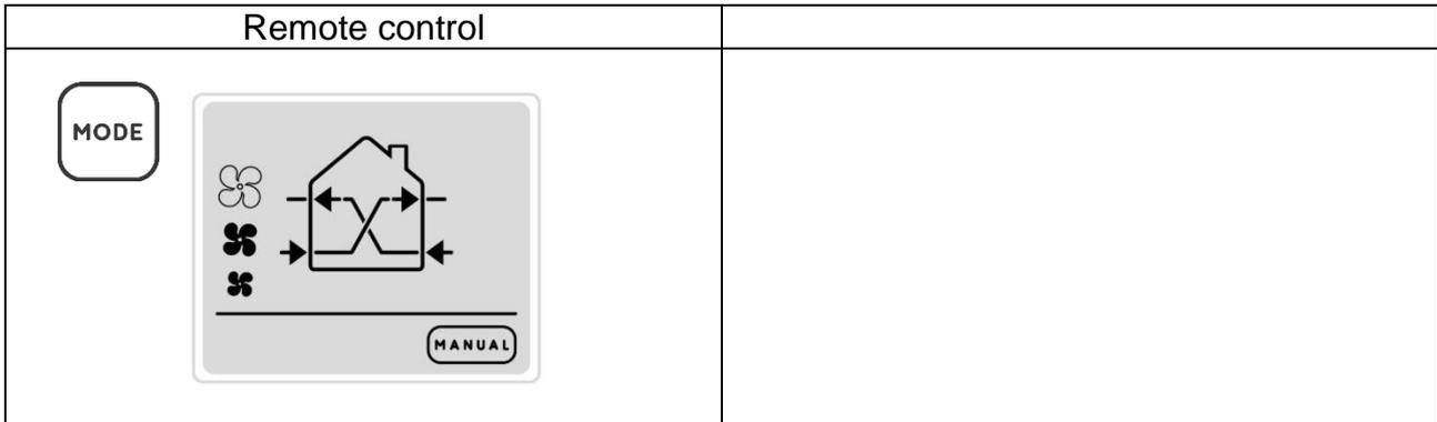
In this mode the sensors are disabled and the units will run with heat recovery. The end user can select the desired speed to run the units and this condition remains until a different command is entered.
