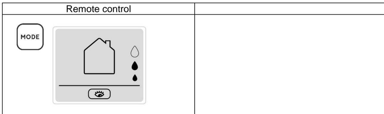
In this mode both humidity and twilight sensors are active, the units will be normally in stand-by with front panel closed, so that when the humidity level in the room exceeds the set threshold the units start running in extraction.
