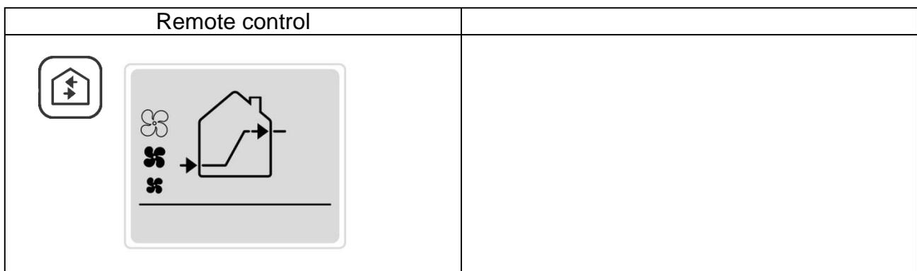
In this mode the units generate a continuous air flow going from MASTER or SLAVE SAME AS MASTER units to SLAVE OPPOSITE TO MASTER excluding heat recovery.
