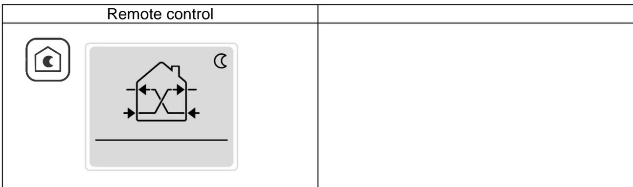
In this mode all the units will run at the night speed with heat recovery until another command is entered.
