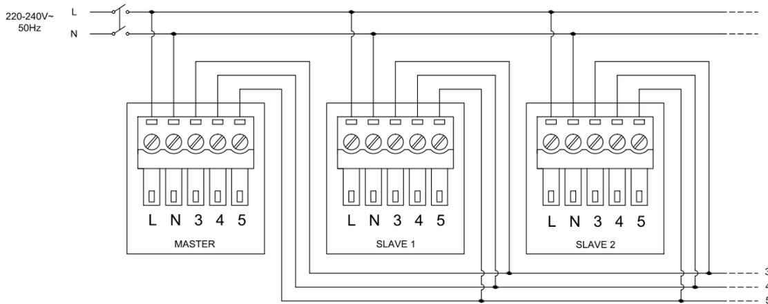
Warning: Humidity and twilight sensors will detect the values from the first unit connected. In case of a system with long wires or with a lot of electric/electronic equipment may cause signal disturbance to use shielded cables and connect a termination resistor of 120ohm on pin 3 and 4 of the terminal block of the last SLAVE.
