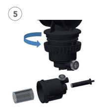
Unscrew the ring nut. Release the body.
