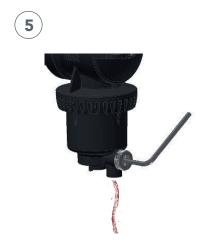
Open the drain. The dirt inside the filter no longer captured by the magnet will be channelled outside by the flow of water in the drain. Use a container of at least 0.5 L.
