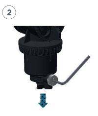
Open the exhaust valve To depressurise the system. (5 Seconds) and close it again. Use a container to collect drain water.
