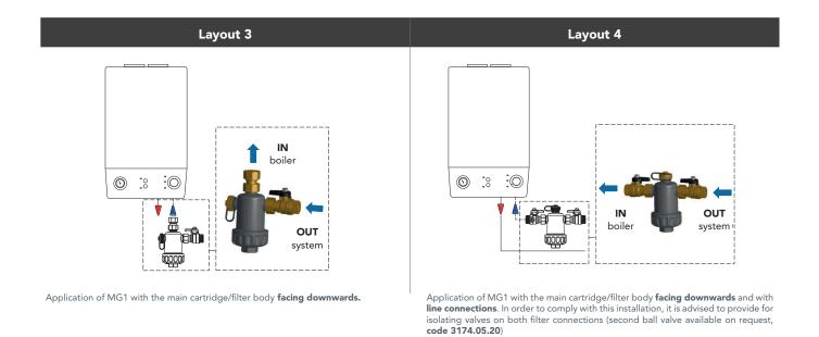
In order to allow the implementation of these installation configurations, it is sufficient to invert the position of the boiler connection swivel fitting and the ball valve (specifically in "Layout 2" and "Layout 4" also the drain cap) and rotate the filter by 90°.
