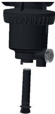
Unscrew the magnet and remove it. Place the magnet on a clean surface.
