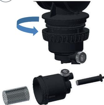
Unscrew the ring nut. Release the body.
