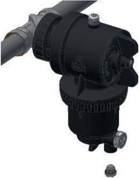
Turn off the pump. Unscrew the drain plug.
