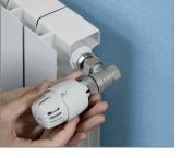
**3.** Position the thermostatic head onto the valve's body by centring the cap's hexagon and leaving the adjustment reference window upwards (in visible position). 4
