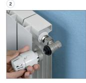
2. Position the polymer spacer onto the valve's body by centring the cap's hexagon (this operation is necessary only for the 3087 series thermostatic head - the spacer is supplied as a kit with the thermostatic head).
