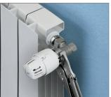
4. Tighten the thermostatic head's knurled metal ring nut onto the valve's body until blocked. Turn the numbered knob a few times after head assembly, from **position "5"** to **position "\*"**, for the parts to settle.
