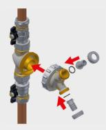
Connect the inlet and drain pipes to the two outlet connectors of the connector itself, open the ball valves and carry out the flushing.
