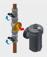
Shut off the device by closing the ball valves and remove the main body of the filter from the diver-
