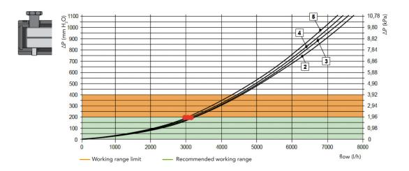
Manifold with "Minipump" ball valve \*
